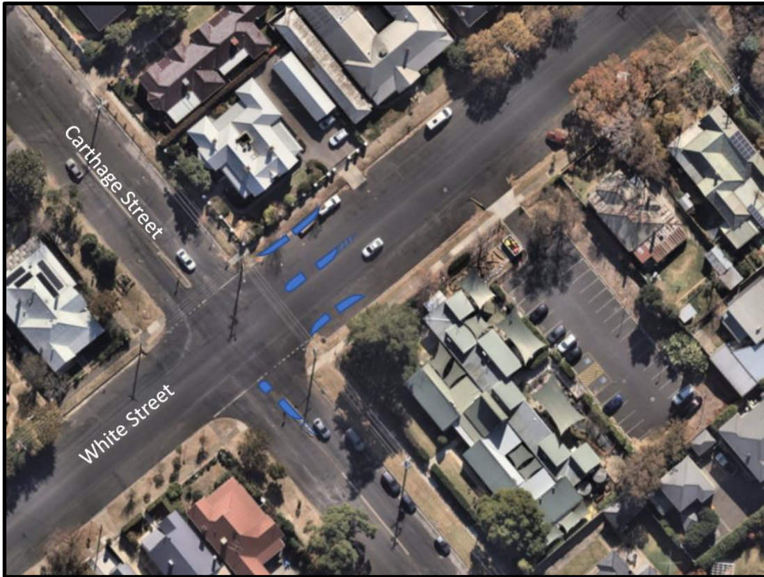
Figure 7: Proposed pedestrian refuges, kerb blisters and line marking at the intersection of White and Carthage Street, East Tamworth
