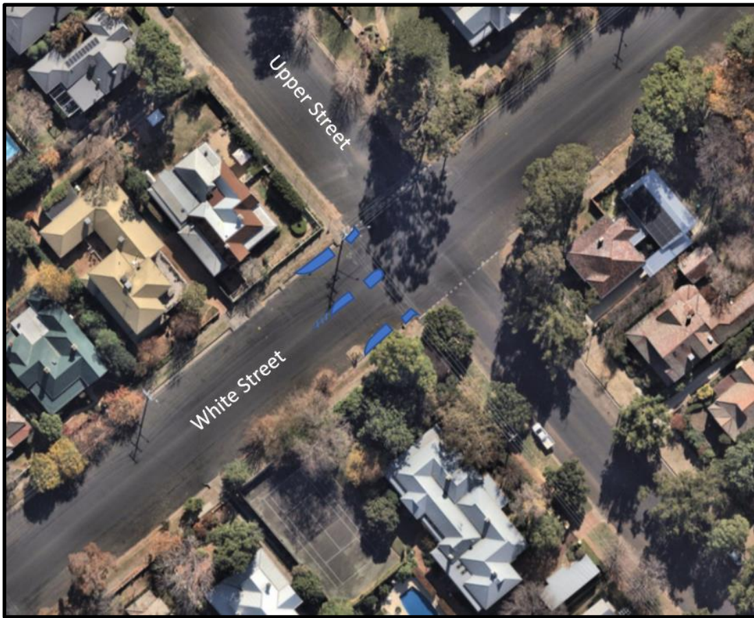
Figure 8: Proposed pedestrian refuge, kerb blisters and line marking on White Street, East Tamworth
