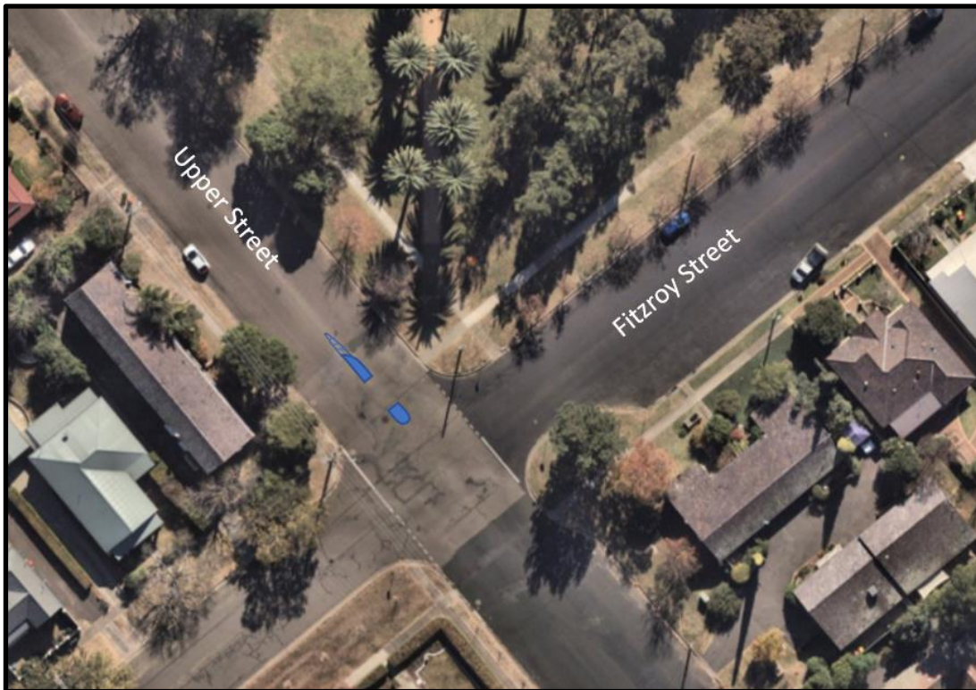
Figure 9: Proposed pedestrian refuge and line marking on Upper Street, East Tamworth
