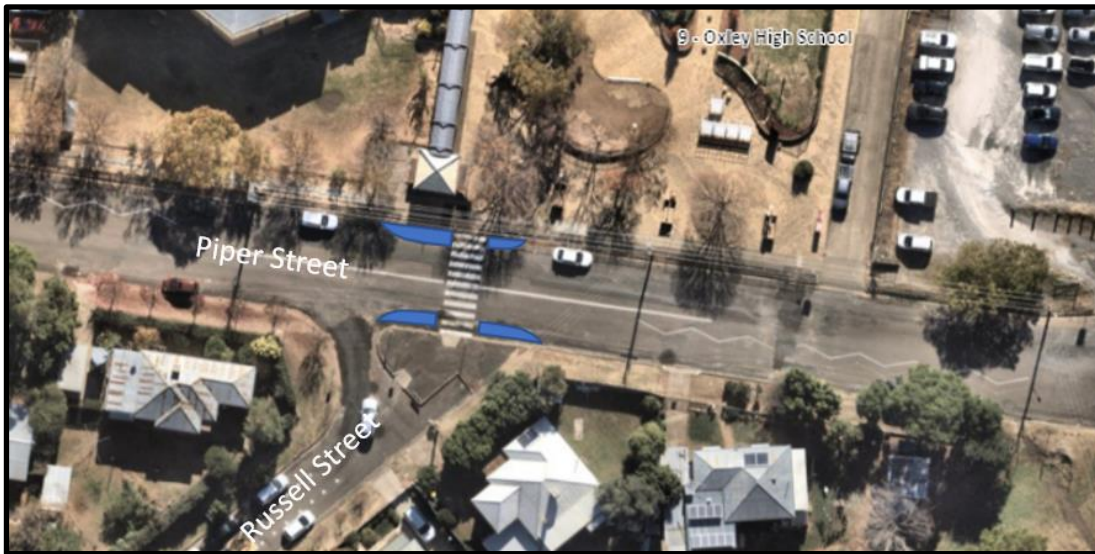
Figure 6: Proposed kerb blisters at Piper Street, East Tamworth
